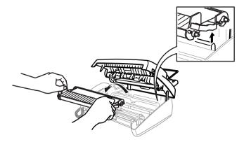
4 To clean the machine's print head, wipe the print head with a lint-free cloth that is dry or lightly moistened with isopropyl alcohol.
